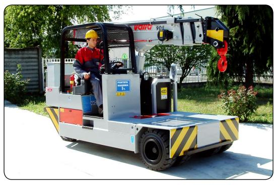
**DRIVE**: DC 10 kW - 48 V fanned, reversible electric motor with MOSFET electronic control HF and energy saving, self diagnostic, speed and temperature checks (2 thermostats), brush wear warning.
